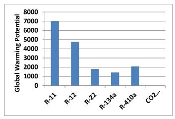
Figure 24. Relative Global Warming Potential of Common Refrigerants
