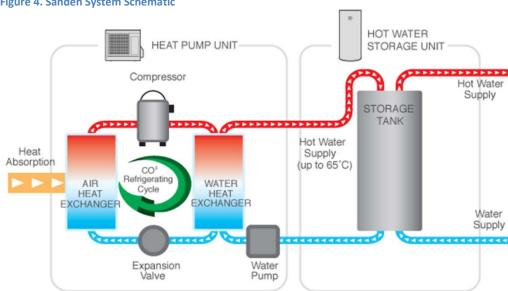
Figure 4. Sanden System Schematic
