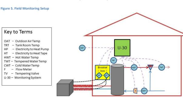
The monitoring collection device is an Onset U30 GSM with cellphone contract so data can be downloaded daily and settings on the logger can be controlled remotely. This quality assurance ensures that issues are identified and corrected as soon as possible. The following monitoring equipment was used:
