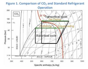
heat from the ambient air as it changes state from a liquid/vapor mixture to a super-heated gas. The compressor then lifts the CO<sub>2</sub> back to the transcritical zone where it transfers heat to the colder water.
